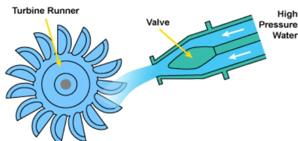
**Fig(1) : Model of Turbine and Water Jet.**
