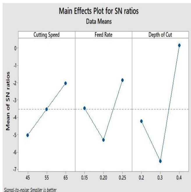
Fig. 1 Main effect plot of S/N ratios for surface roughness
