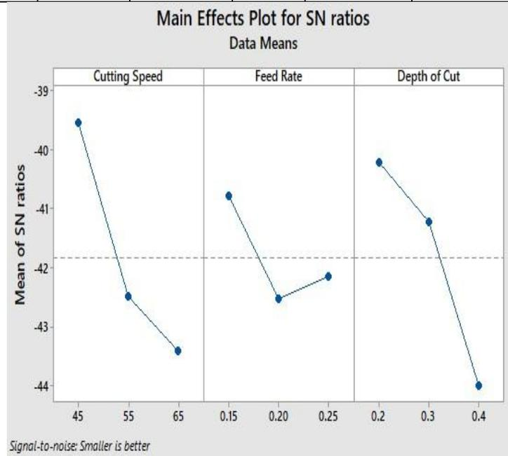
**Fig. 2 Main effect plot for S/N ratios for cutting force**
